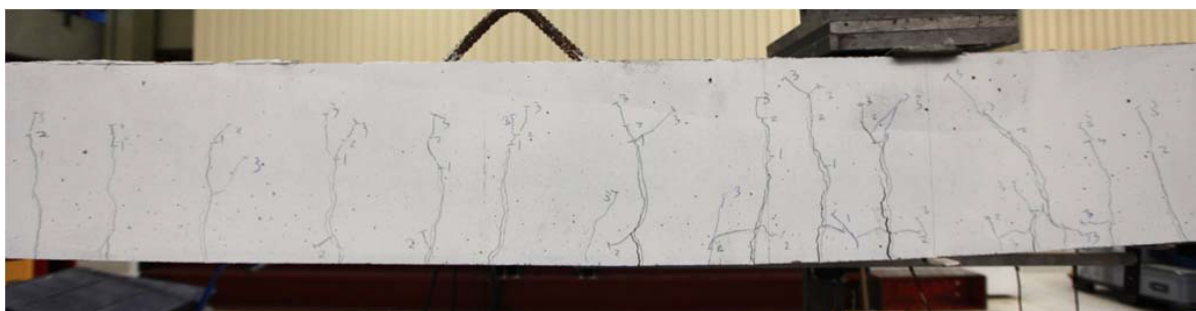
Figure 4.10: Observed experimental failure crack pattern in C451A2
