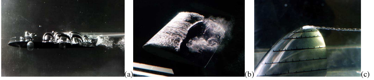
Figure 9. Cavitation. (a) Bubble cavitation, (b) sheet cavitation with emerging cloud cavitation and (c) tip-vortex cavitation. Images from http://www.fluidlab.naoe.t.u-tokyo.ac.jp .
