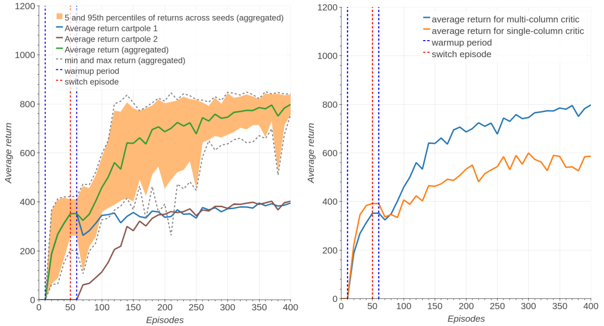
Figure 5-3: Learning curve for the flexible DDPG algorithm with a multi-column Critic architecture (left), and a comparison with a single-column architecture. In all experiments the actor architecture was also multi-column. It can be seen that the multi-column critic architecture converges quicker to an optimal policy, because each stage (and thus cartpole) in the curriculum has access to it's own parameters. The only difference with a decentralized approach is that the Critic still outputs one Q-value, because it only has access to the aggregated reward signal.
