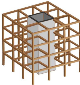
Figure 1.2: Concrete core with timber frame structure.
