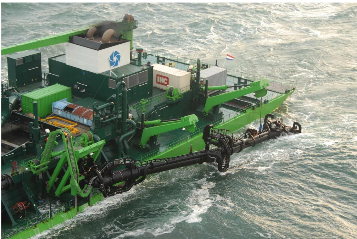
Figure 2.6: The suction pipe hoisted with gantries, source: [?]
