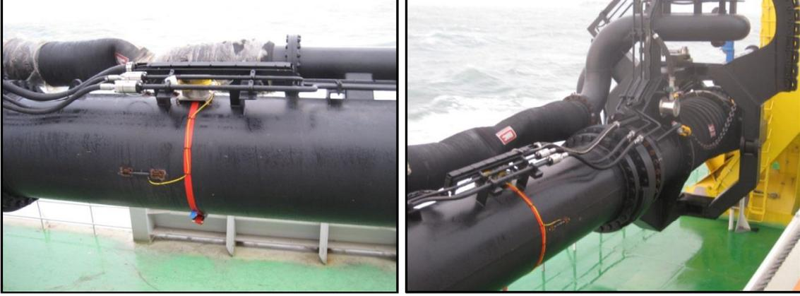
Figure 3.14: Mounted force sensors on the suction tube of the TSHD: 'Chang Jiang Kou', source: IHC
