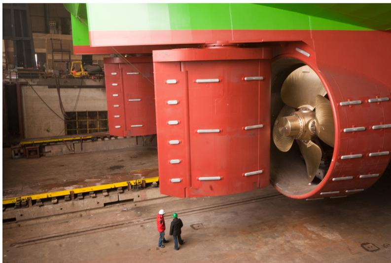
Figure 2.2: Controllable pitch propellers and rudders of the Congo River, source: [?]
