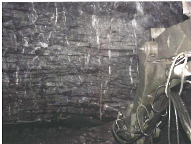
Figure 5.11: Horizontal stress induced fractures above the back of the previous cut in cut and fill mining in the A zone. (Nyström, 2005a)
