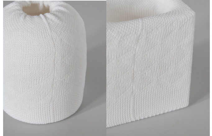
Fig. 5.21: Visible connection lines in sock 9.
