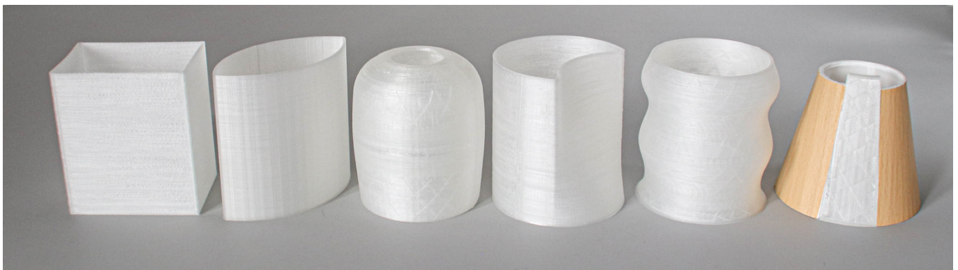
Fig. 5.18: Shapes of the Socks & Cylinders experiment. From left to right: rectangular, flattened cylinder, spherical, convex-concave demo, wobbly and conical shape.
