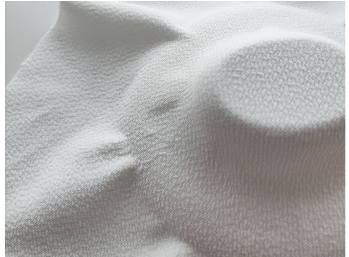
Fig. 5.16: Non-developable surface with air bubbles caused by the textile not being glued to the surface sufficiently.
