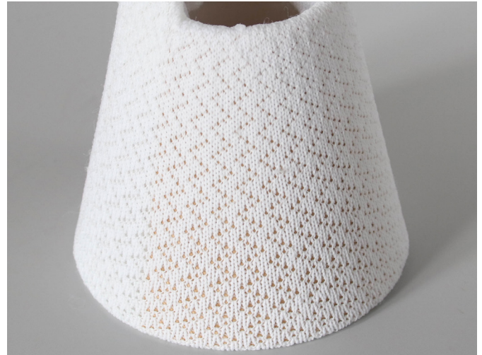
Fig. 5.25: Visible differences in the pattern at the bottom and top of the conical surface. It is slightly warped.
