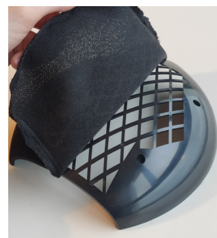
Fig. 3.34: No glue on the surface (JBL CS460 sat).
