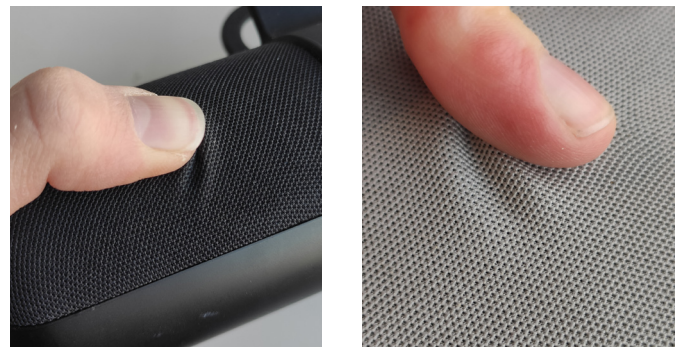
Fig. 3.31: Movable fabric over the surface of the Miniso speaker and Bose Soundtouch.
