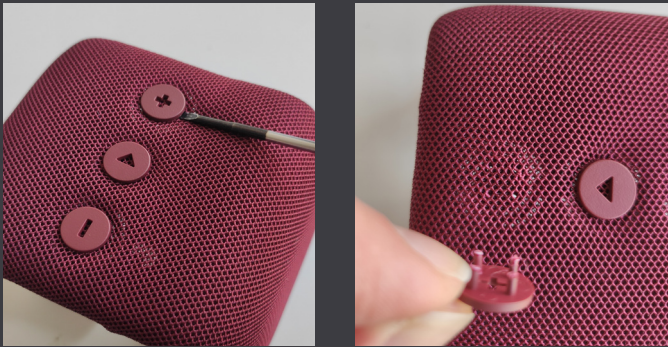
Fig. 11.4: Outside surface of Fresh 'n Rebel Rockbox Bold S: button with pins can be popped off.
