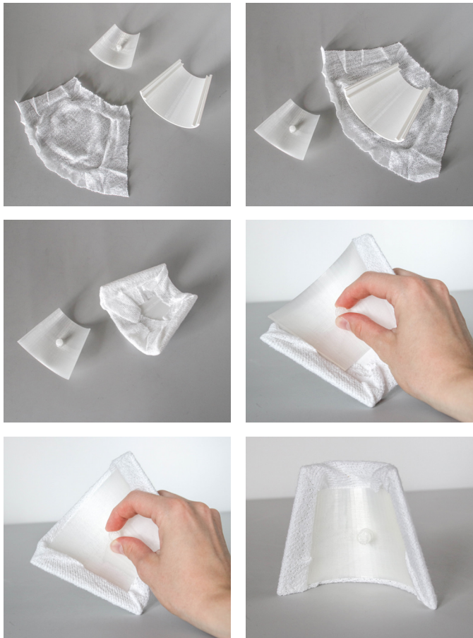
Fig. 6.19: Assembly steps of the clamp system.
