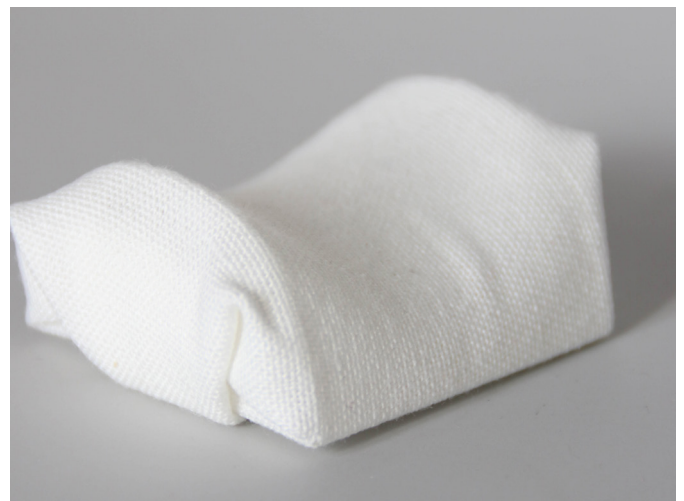
Fig. 5.14: Shallow saddle shape covered with woven textile. Air bubbles are visible because the textile is not glued to the surface.
