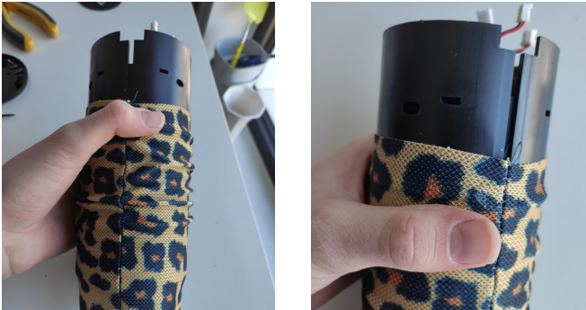
Fig. 3.35: Leopard printed speaker with sewn sleeve: inner housing contains a slot for the seam allowance.
