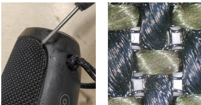
Fig. 4.27: Blue and yellow yarns create a black fabric.
