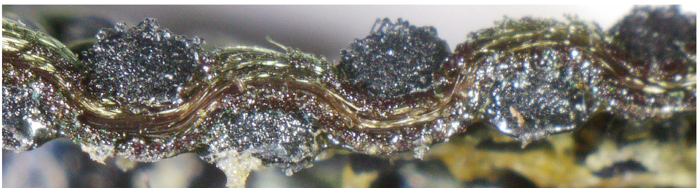
Fig. 3.26: Cross-section of the fabric, where the integration of thick and thin yarns can be observed.
