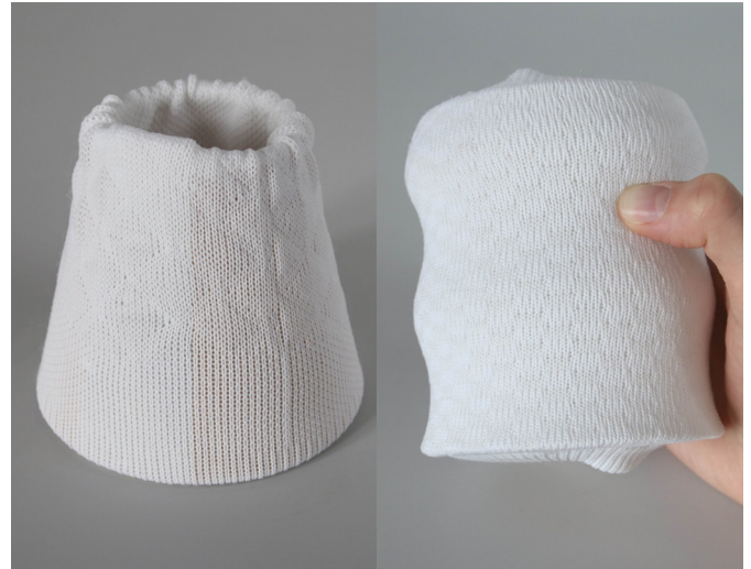
Fig. 5.19: On the left: sock 9 is not tight enough around the top of the cone. On the right: sock 1 is too tight and stretches over the smallest diameters.
