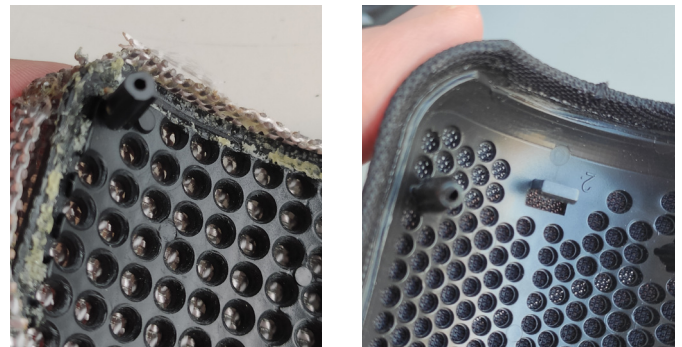
Fig. 3.30: Glued inner edges (left) and welded edges (right).
