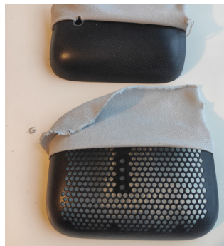
Fig. 3.23: Non-developable surfaces of the Google Nest Audio.
