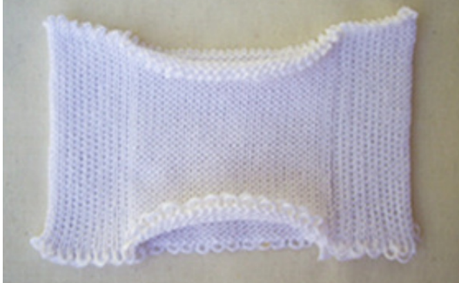
Fig. 4.23: Tube with flange, made on automated flatbed knitting machine (Underwood, 2009).
