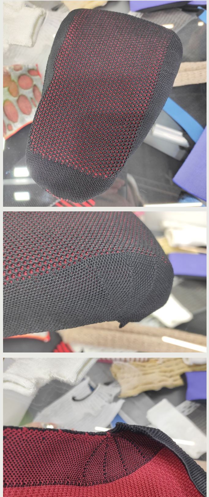
Fig. 4.10: 3D-knitted seat cover by Stoll flatbed knitting machine. Pictures made by the author at TechTextil 2022.
