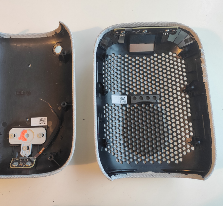
Fig. 6.1: Google Nest Audio with textile glued to the outer- and inner surface.
