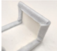
Folding at the inner edges of the felt.
