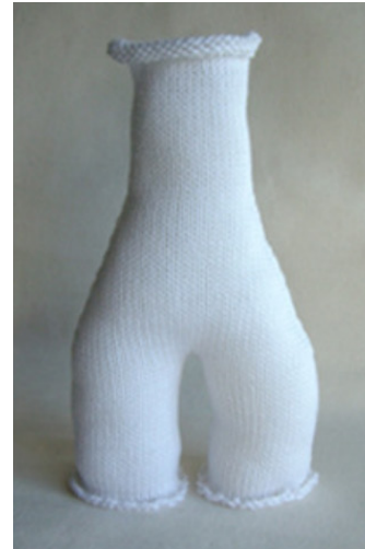
Fig. 5.24: 3D-knitted example of a complex continuous shape that can be made on a flatbed knitting machine.
