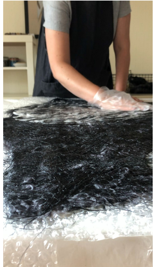
Fig. 4.5: Felting done by hand with the use of soap.
