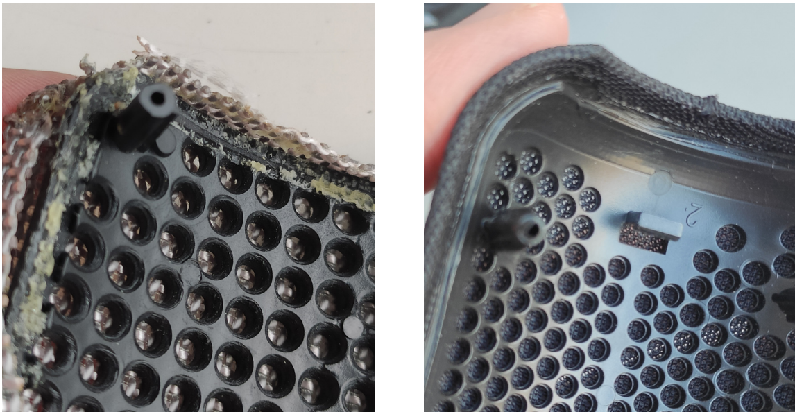
Fig. 6.2: Glued textile housing with visible glue (left) and welded part with no observable glue (right).
