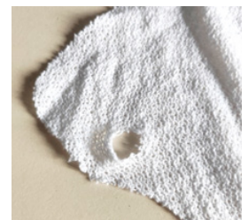
Holes in the fabric of prototype 2 are stretched out.
