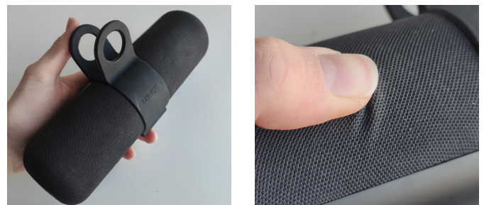
Fig. 6.5: Miniso speaker with fabric that can shift over its surface.
