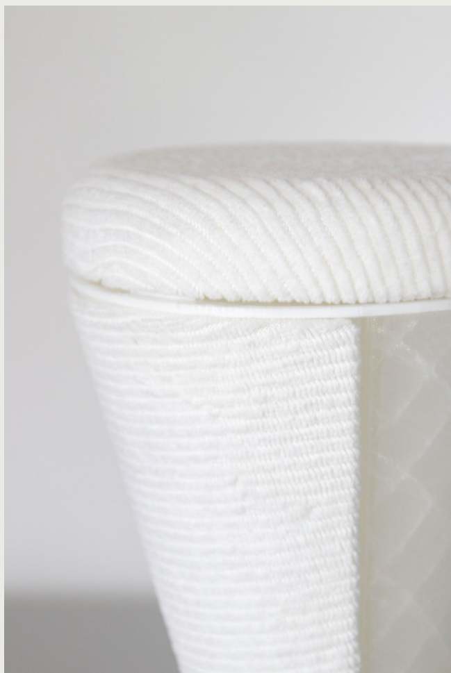
Fig. 4.31: Corduroy and spacer fabric parts attached to the Rotation Lamp prototype.
