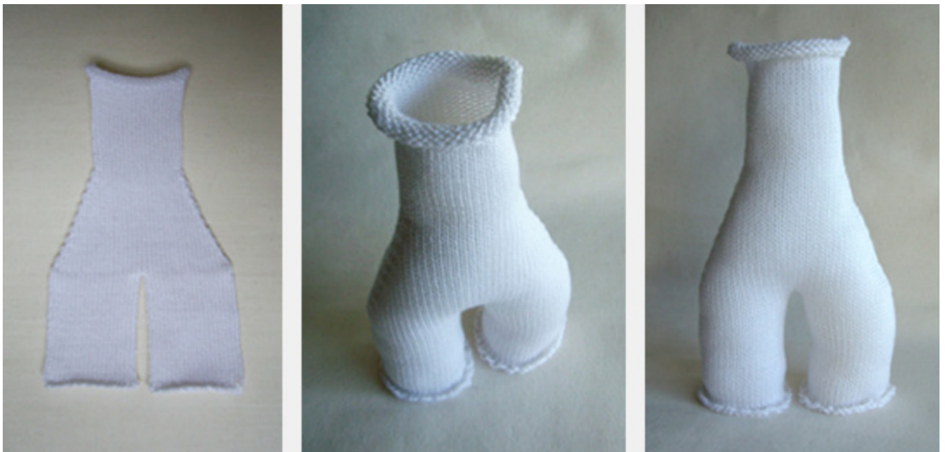
Fig. 4.24: Y-shaped textile, made on automated flatbed knitting machine (Underwood, 2009).
