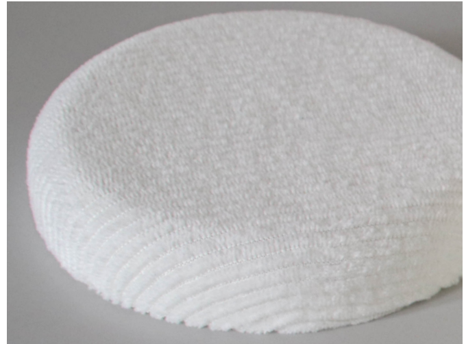
Fig. 5.12: Example of a flat surface covered with knitted corduroy fabric. This shape is non-developable, however it resembles flat surface coverage as well.
