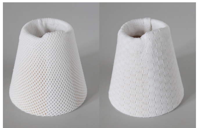
Fig. 5.22: Comparison of diagonal and horizontal-vertical patterns on the conical shape.
