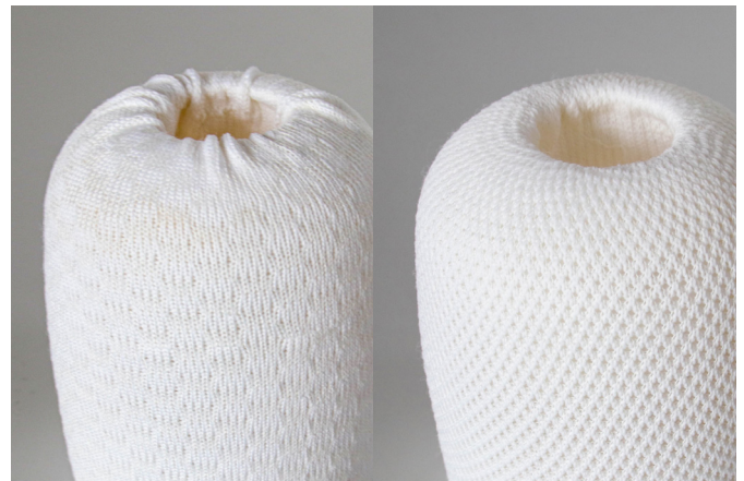
Fig. 5.26: Not all socks allow tucking inwards without folding. The sock on the right works because of its open knit structure.
