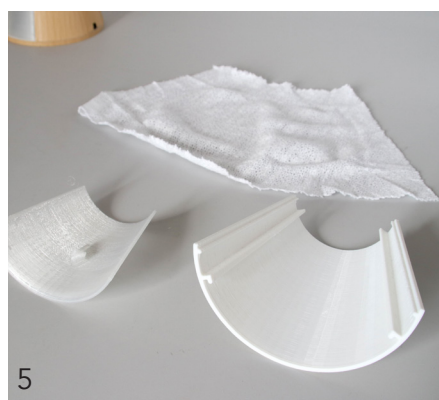
The textile and housing materials are separated for accurate recycling of separate waste streams.
