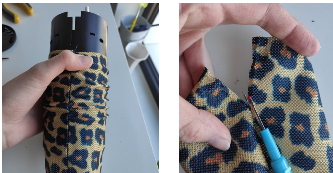
Fig. 3.17: Sewn sleeve of the leopard speaker. Non-developable surface.
