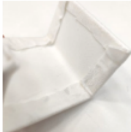
Thin fabric: does not accumulate in inner edges
