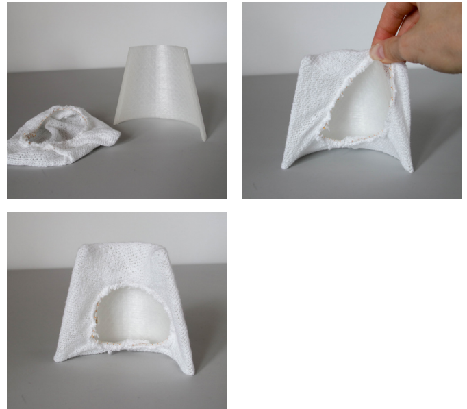
Fig. 6.20: Assembly steps of the cover system.
