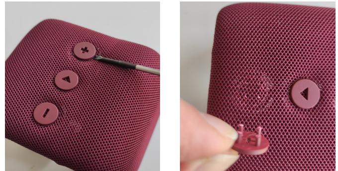
Fig. 3.38: Outside surface of Fresh 'n Rebel Rockbox Bold S: button with pins can be popped off.
