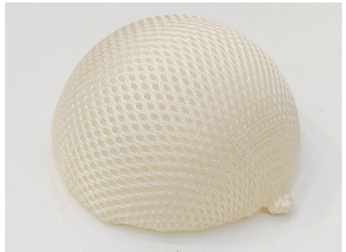
Fig. 5.15: Spherical shape covered with knitted stretchable spacer fabric.
