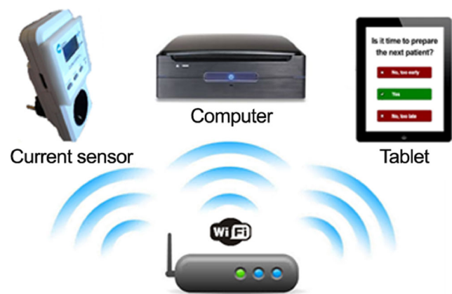
Fig. 2 Schematic overview of the real-time prediction system
