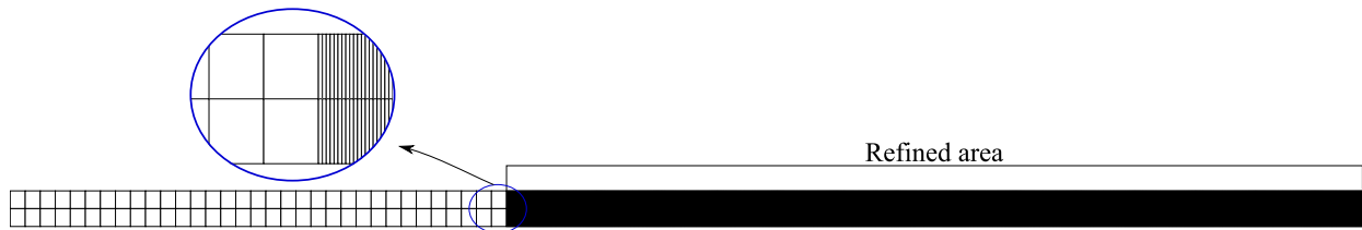
Fig. 13. Mesh of the reference model used for the performance and accuracy comparisons. Remark that the thickness of the specimen varies for some of the numerical tests.
