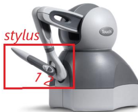
Figure 3 - The Phantom Omni ( https://www.3dsystems.com/haptics-devices/touch ). The stylus is the pen-like device inserted into the device when not used. The 1 and 2 indicate the buttons that are located on this stylus. Button 1 is the one on the back (white/light) and button 2 is the one on the front (black/dark).
