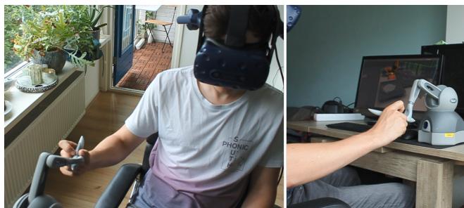
Fig. 1. Pictures of the experiment setup. The participant is holding the stylus of the Touch haptic device and is wearing the HTC Vive HMD.
