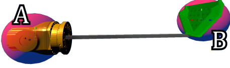
Fig. 3. The scoop attached to the industrial robot. The two red spheres show the locations for which the VFs are activated where A is the wrist joint and B is the scoop. The green volume, consisting of small spheres near location B represent the voxels that are used to approximate the submerged volume of the scoop.
