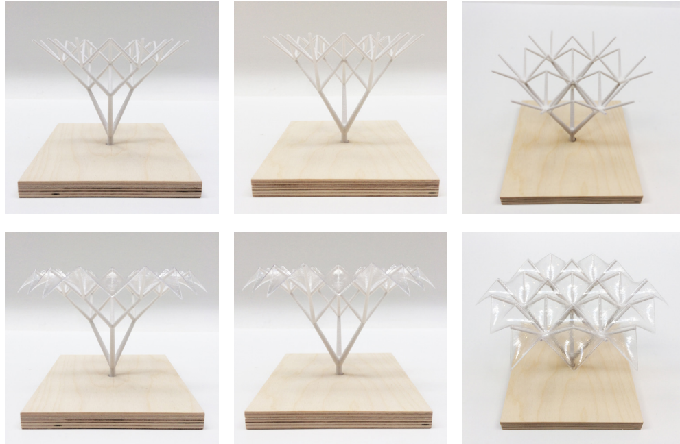
[198] SINGULAR 3D PRINTED GYPSUM BRANCHING STRUCTURE WITH VACUUM FORMED ROOF
