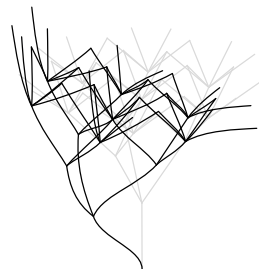
DEFORMATION BY DEADLOAD + WINDLOAD
