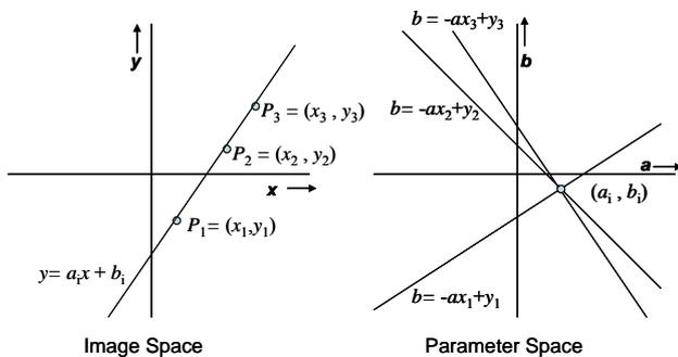
Figure 1. Hough transform for lines in 2D
