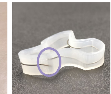
Figure 9.12 The ends of the wires not attached to each other and were not able to be aligned.
