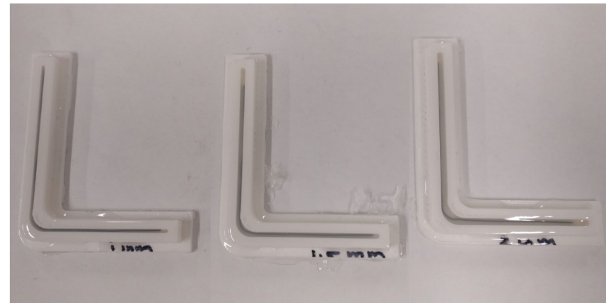
Figure 9.8 The 3D-printed molds filled with A50 silicones and SMA wire of 0.5mm. Thickness of the mold from left to right: 1mm, 1.5mm, and 2mm.
