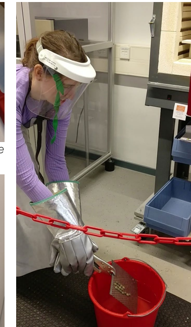
Figure 6.12 Process of taking out the metal plate with safety gear.
