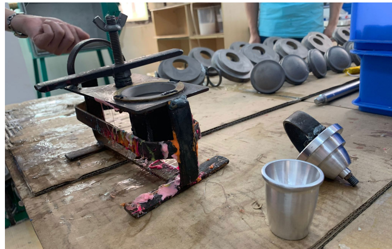
Figure 6.5 Prototype of the 4 part mould of the Beppy Cup. The core parts are on the right
