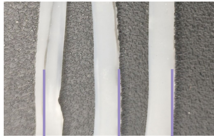
Figure 9.9 Different position of wire in 1mm, 1.5mm, and 2mm thickness cast.
