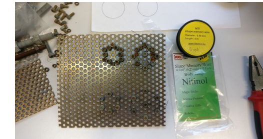
Figure 6.10 SMA wires fastened between the plate and the screw.
