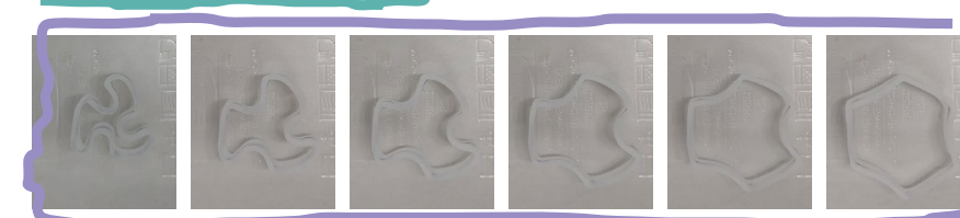
Figure 9.14 Composite of SMA 0.5mm wire and A50 shore silicone reacting with hot water returning to its original hexagon shape
