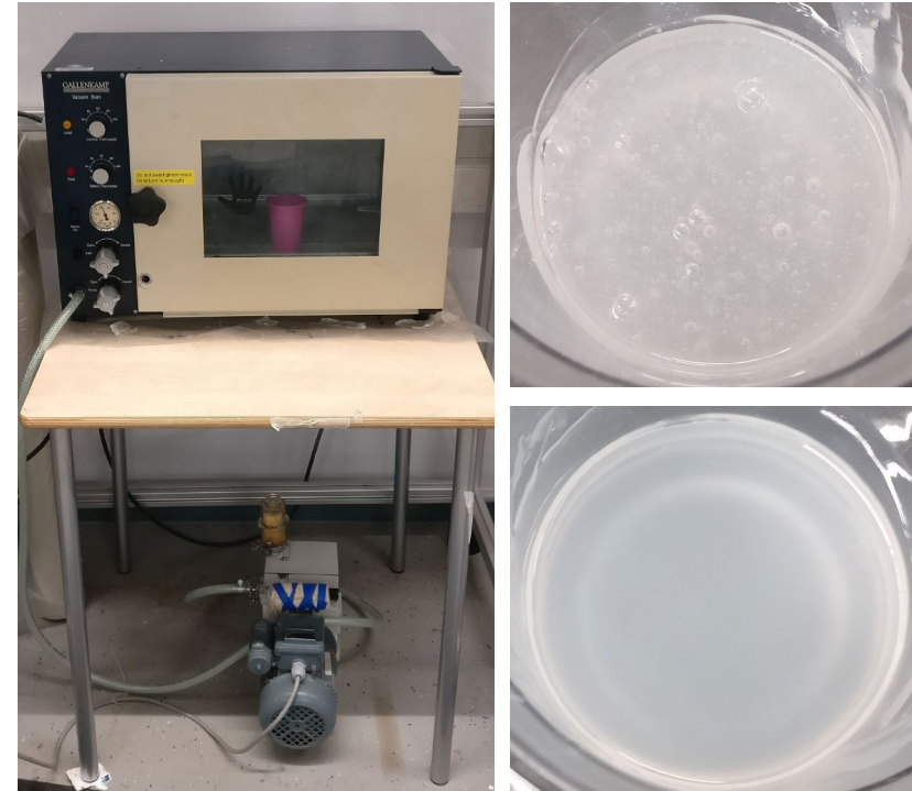
Figure 9.21 Vacuum chamber (left) and silicone cup before with all the air bubbles inside (top right), and after being in vacuum (bottom right)
