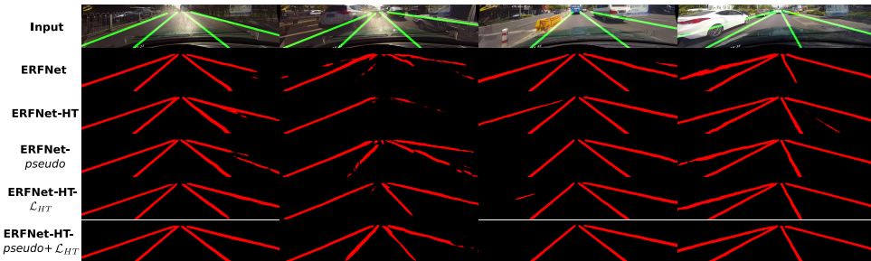
Figure 3.2: Visualizations of predicted lanes on the CULane dataset. Only 10% annotated data is used for training. ERFNet-HT- pseudo + \mathcal{L}_{HT} performs better on challenging samples and better localizes lane boundaries. The inference speed of the ERFNet-HT is around 13 frames per second on a NVIDIA GTX1080Ti GPU.
