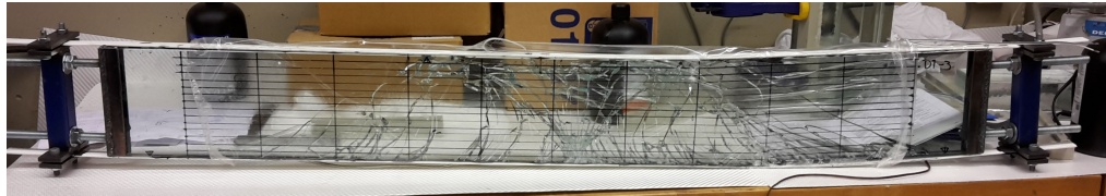
Figure 6.18: Crack pattern of failed specimen BEN1-PT-2
