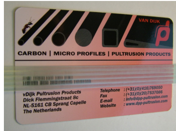
(a) Transparent GFRP strips produced by DPP
