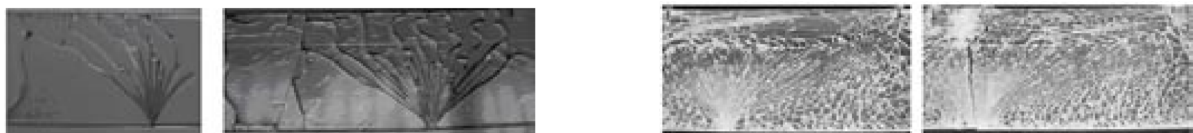
Figure 2.13: Cracking patterns of annealed and fully tempered glass pane due to bending, by Veer et al. [2005]
