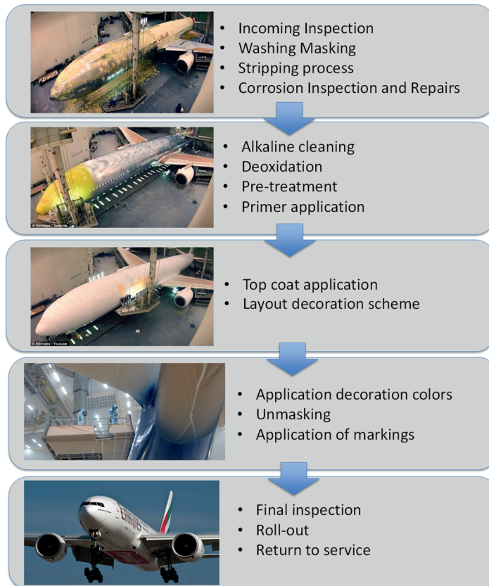
Figure 2.11 Steps required for aircraft painting (images kindly provided by Airbus and Emirates Airlines).
