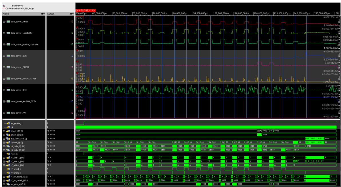
Figure 5.13: Time based power consumption graph of individual NPE operations.
