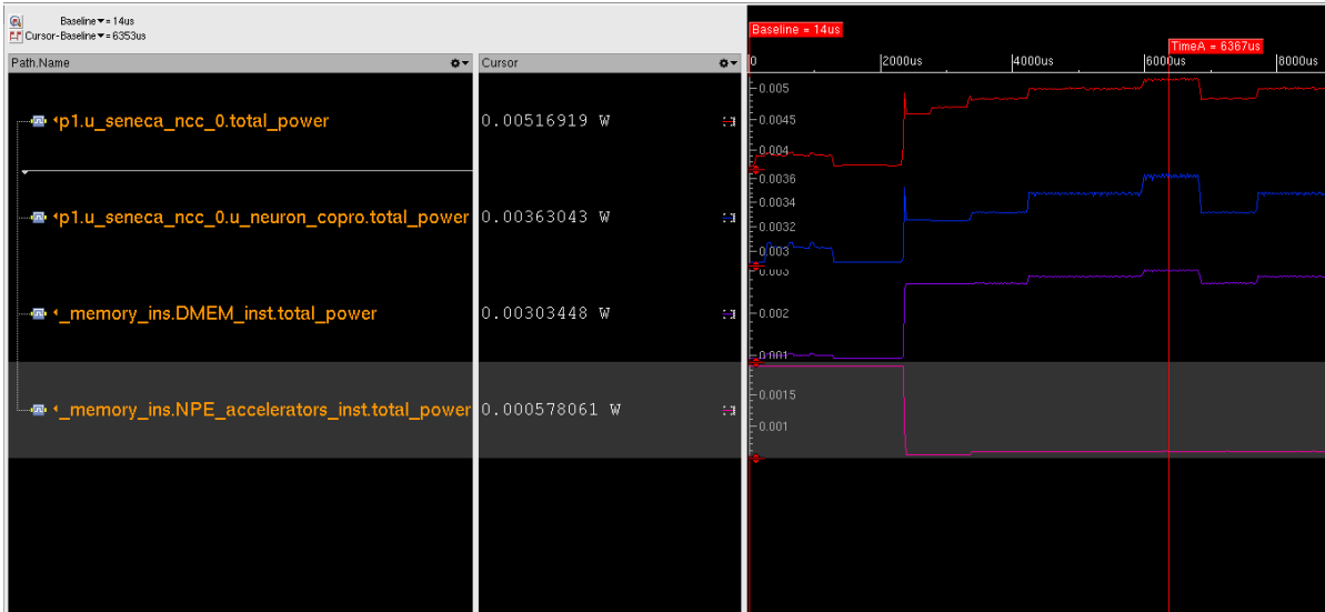
Figure 6.3: Time-based power graph of version 3, broken down into components (core 1).
