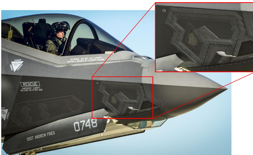
Figure 1.2: Nose of the Lockheed-Martin F-35A, showcasing composite panels with functional material inserts on their edges
