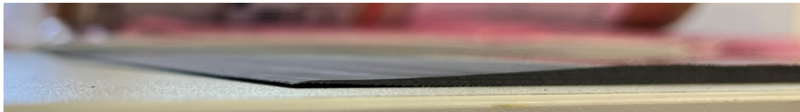
(c) Curvature of the scarf edge of a laminate
