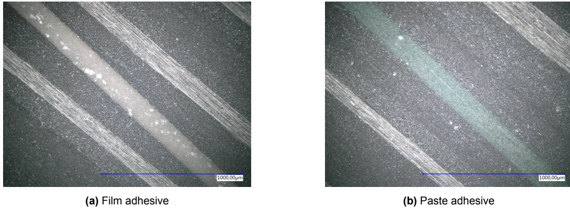
Figure 7.5: Micrographs showing the bondline of the MCLS specimens
