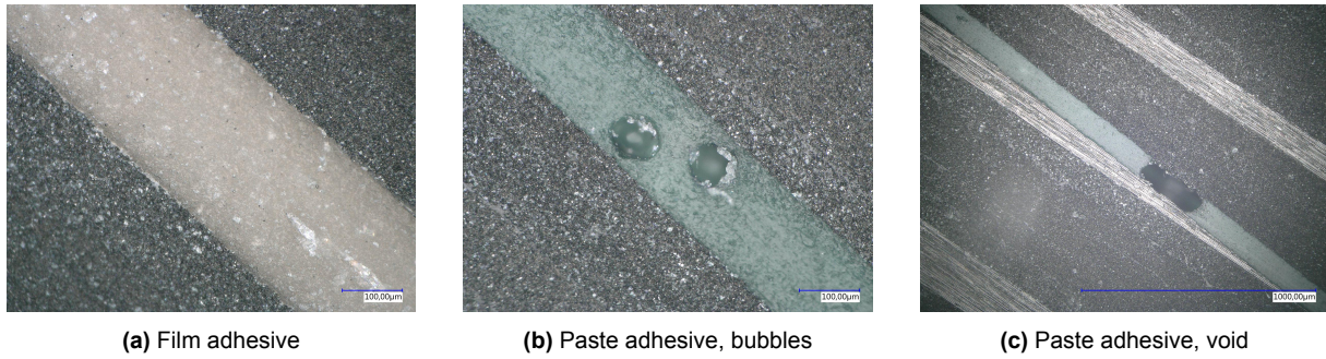
Figure 7.12: Micrographs depicting imperfections — or the lack of — in the bondline of the MCLS specimens
