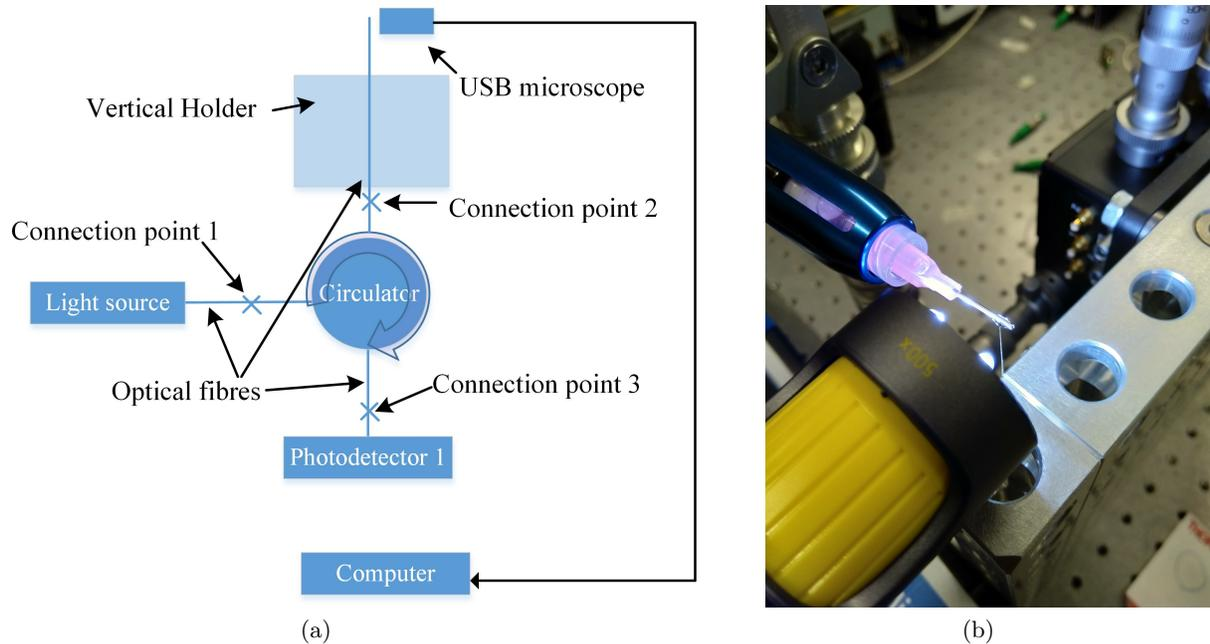
Figure 3: Experimental setup (a) Structural diagram; (b) Photo of the optical fibre end
