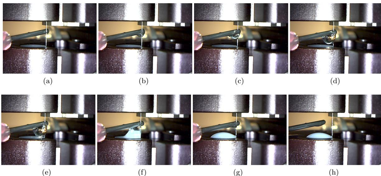
Figure 9: The process of dropping liquid on optical fibres (a)-(h) are the photos of dropping liquid process in a sequence
