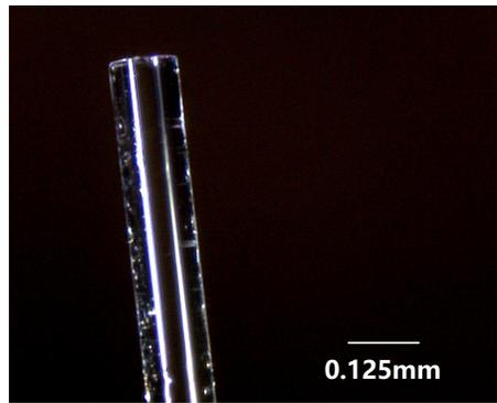
Figure 4: A close look of the end optical fibre from USB microscope
