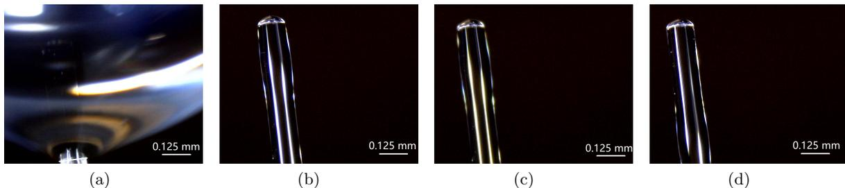
Figure 5: The process of dropping liquid to the end of optical fibre (a) forming droplet on the end of optical fibre; (b)-(d) three instantaneous status of after dropping liquid on the end of optical fibre
