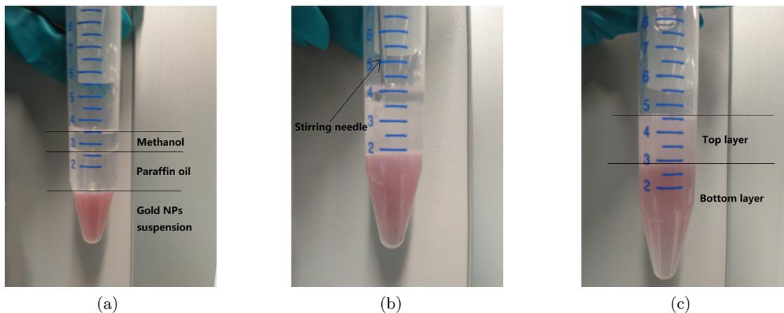
Figure 2: The process of transferring Gold NPs from citrate buffer to paraffin oil (a) Photo taken before stir without stir needle; (b) before stirring with the needle; (c) after stirring
