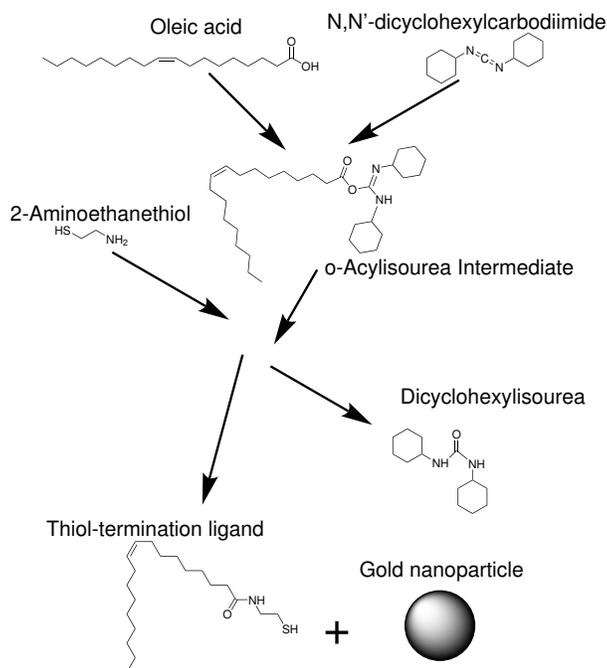
Figure 1: The process of generating gold nanoparticles with thiol-termination ligand based on the method of López-Millán et al.<sup>9</sup>
