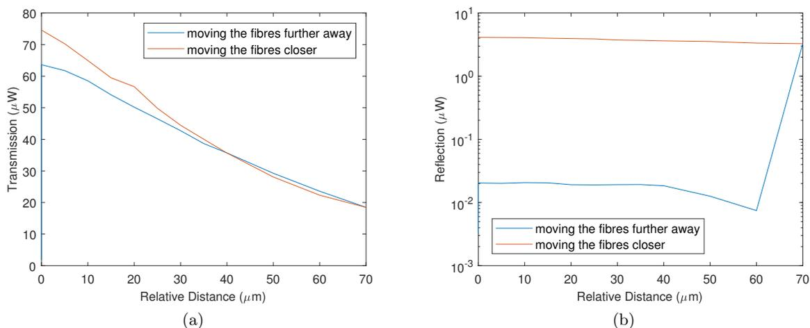
Figure 10: Moving optical fibre with refractive index liquid (a) Transmitted light; (b) Reflected light
