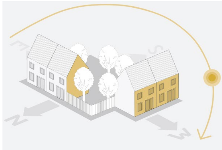
Figure 12: Solar exposure for different building orientations (Richards Partington Architects, 2012).
