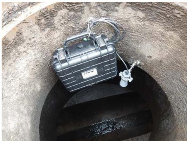
**Figure 11.23** LoRaWAN prototype including water level sensor (MaxBotix) installed in a sewer manhole. *Source:* Eawag.
