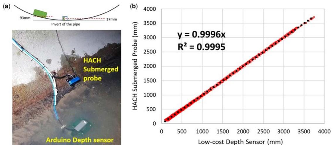
**Figure 11.15** Arduino and HACH sensors installation location inside an urban stormwater drain; (a) The water level readings of a rain event; (b) Correlation between Arduino and HACH sensors. *Source:* EPHM Lab and BoSL.
