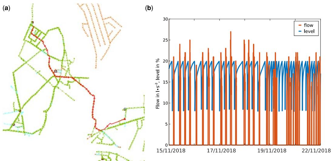
**Figure 11.11** The change in the dry weather pattern in a pumping station is traceable 3.5 km downstream in a downstream flow monitoring location; (a) flow path between discharge point and monitoring location; (b) change in patterns recorded on 19/11/2018. *Source:* Aquafin NV.
