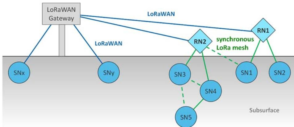
**Figure 11.25** Synchronous LoRa mesh topology (RN: repeater node; SN: sensor node). Dashed lines between synchronous LoRa mesh sensor nodes indicate alternative link paths. *Source:* adapted from [Ebi et al. \(2019\)](#).
