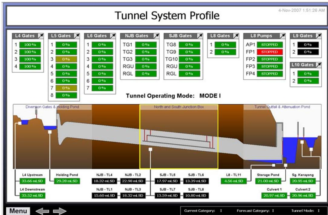
**Figure 11.7** A snapshot of operational display Mode 1, showing the operational status of the gates installed along the tunnel. Note: NJB and SJB gates are for the traffic tunnel. *Source:* Department of Irrigation and Drainage, Malaysia.
