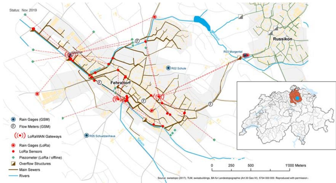
**Figure 11.20** Overview on the UWO sensor network in Fehraltorf including sensors and low-power wide-area network (LPWAN) infrastructure (Status: November 2019). Small figure: location of the Canton Zurich and the case study location, 12 km north-east of the city of Zurich within Switzerland. *Source:* Eawag.
