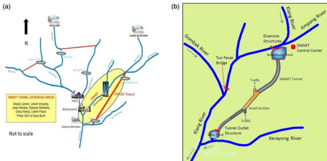
**Figure 11.2** The location of SMART Tunnel alignment (a), diverting the discharge from Klang/Ampang Rivers to Kerayong River (b), minimizing flood occurrence within the marked SMART coverage. *Source:* Department of Irrigation and Drainage, Malaysia.
