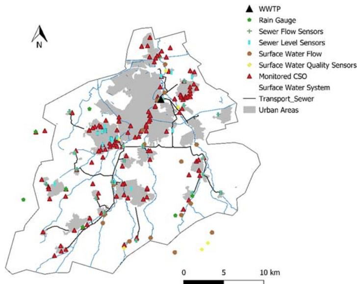
**Figure 11.1** Monitoring network for Dommel River and Eindhoven urban drainage system. *Source:* Job van der Werf (TU Delft).
