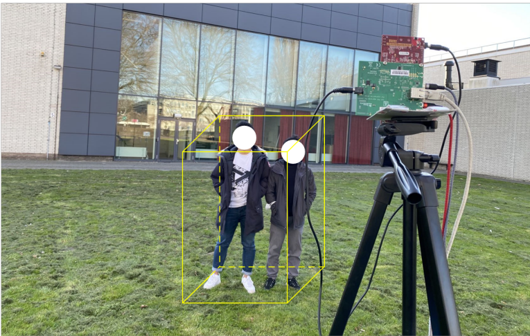
Figure 3.1: The ground truth of Group People with 2 individuals and the FMCW MIMO Radar is used.
