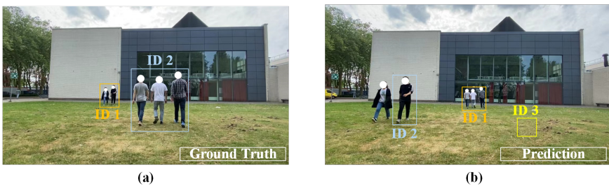
Figure 5.3: Example of calculating MGTA. (a) People Counting scenario in the real world (ground truth) at t_1 . (b) Predicted identities of groups from tracking for counting methods at t_2 .
