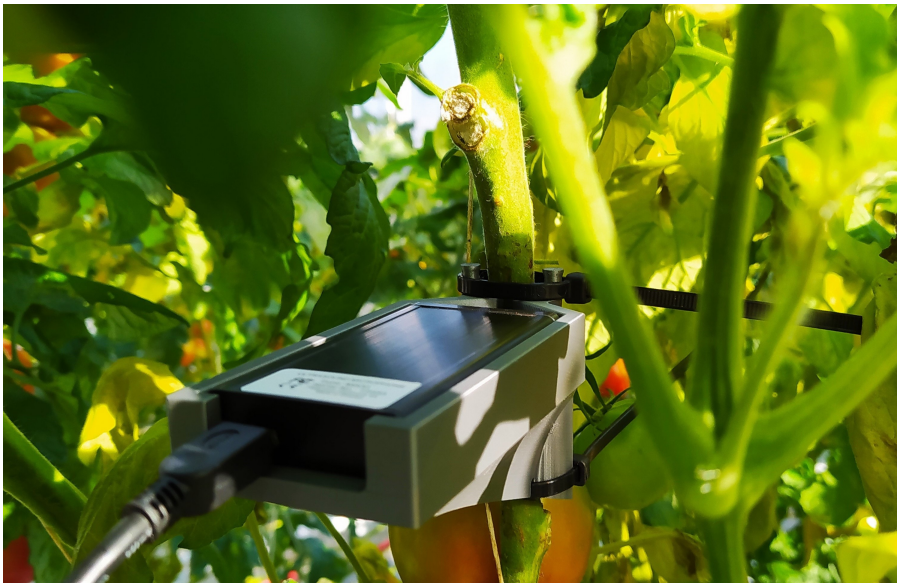
Figure 26: The first prototype of our passive ultrasound sensor module
