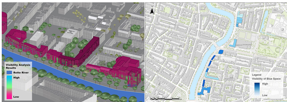
Fig. 4: Building-based visibility analysis results: Visualizing in Rhino (left) and summarizing on map (right)
