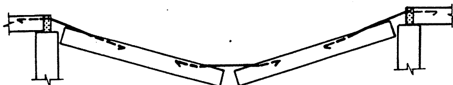
Figure 3.13: Catenary action in a precast floor with torn out ties due to transverse forces
