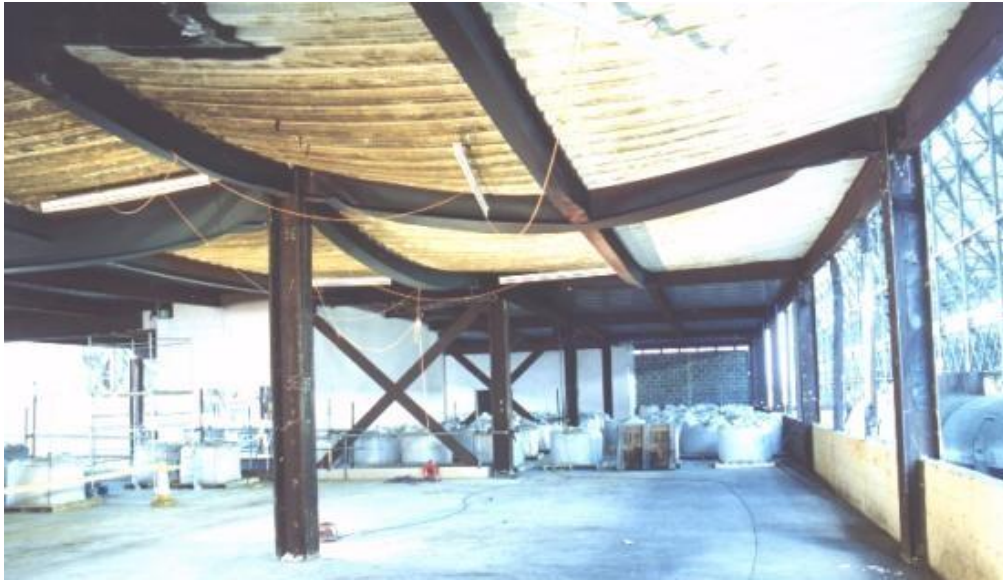
Figure 27 Fire-induced permanent sagging of a composite steel structure (Cardington fire test) (54)
