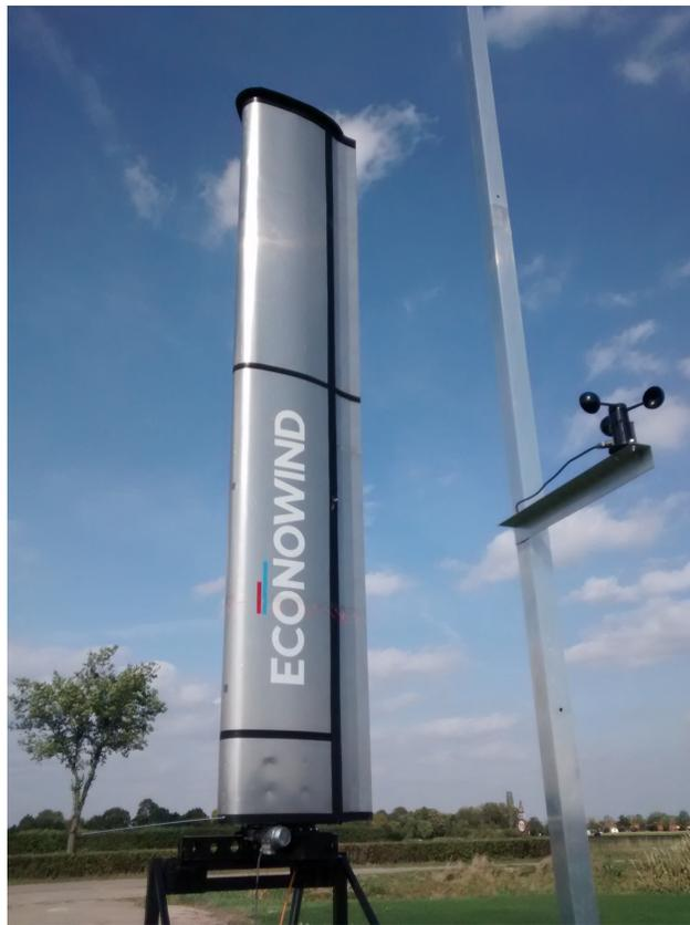
Figure 1.10: Measurements on the VentiFoil half scale model
