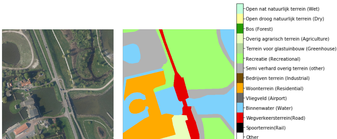
Figure 3.2: Example of a 480 \times 480 aerial image patch (left) and corresponding annotation (right).
