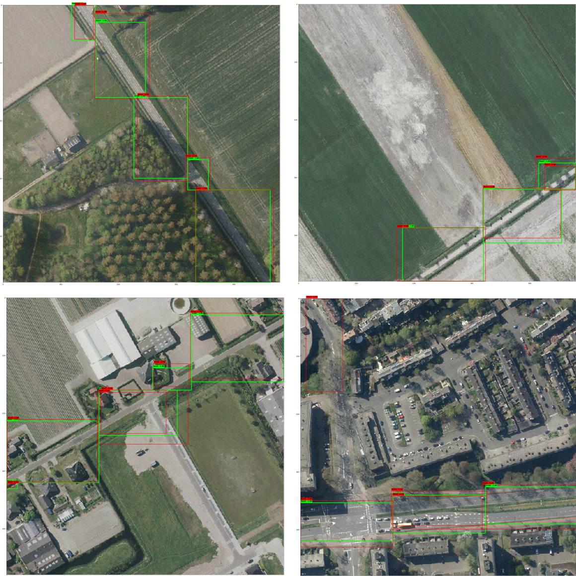
Figure 4.10: Aerial images with predicted localizations of road segments and annotated localizations. Red boxes are predictions, whereas annotated boxes are displayed in green. The values near each box display the confidence of the prediction of the box, which 1 for all annotated boxes.
