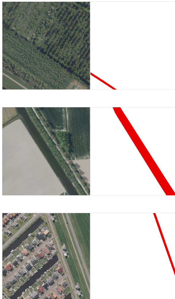
Figure 4.17: Seemingly inconsistent road width annotations of three samples of aerial images with their corresponding annotations. Roads are depicted in red on the annotations.
