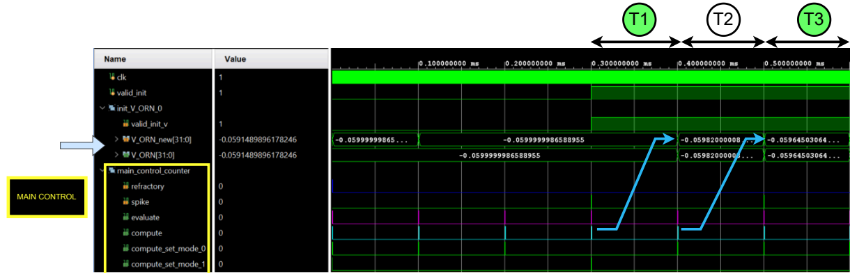
Figure 4.12: Updating V[t + \Delta t] in timesteps of 0.1 ms using the Voltage Update and Storage Module .
