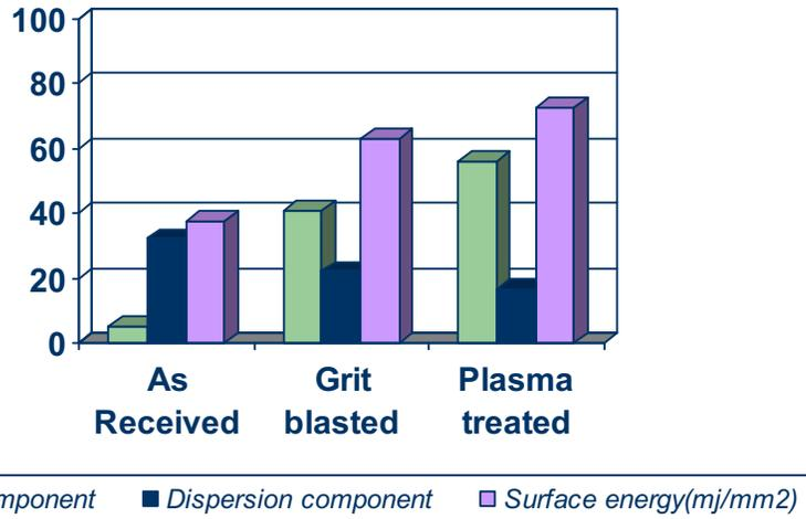
**Figure (1) Surface energy estimation of titanium after different treatments.**
