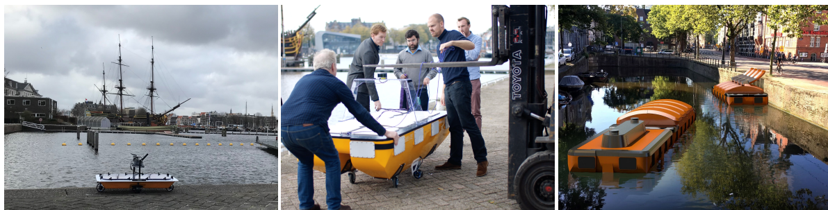
(a) 1:4 scale Roboat on the quay in Amsterdam near AMS Institute (b) 1:2 scale Roboat just before going into the water ©2019 AMS Institute (c) Render of full scale Roboat transporting a dumpster ©2018 Pietro Leoni
