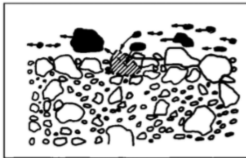
Figure 4.5: A schematic of vertical winnowing of finer material given by Parker and Klingeman (1982) . Flow is from right to left.
