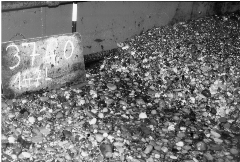
Figure 2.4: Gravel dune at the study reach photographed inside the diving bell of Carl Straat vessel (image courtesy: WSA, BfG).
