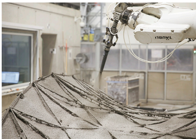
FIGURE 10 left: Robotic shotcrete process, right: Surface quality after shotcrete.
