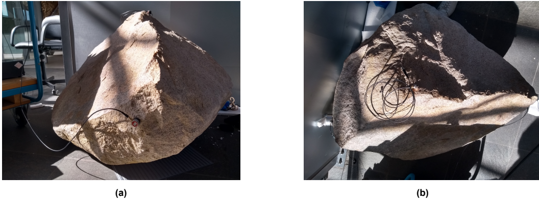
Figure 11.4: Setup of reflection test for hammer from top (a) and from 'bottom' receiver (b) on a granitic rock.
