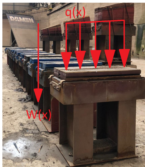
Figure 3.2: Dock block modelled as a component that is designed to support transverse loads ( q(x) ), that is, loads that act perpendicular to the longitudinal axis of the beam. The beam supports the load by bending only and lead to a deformation W(x) along this longitudinal axis.
