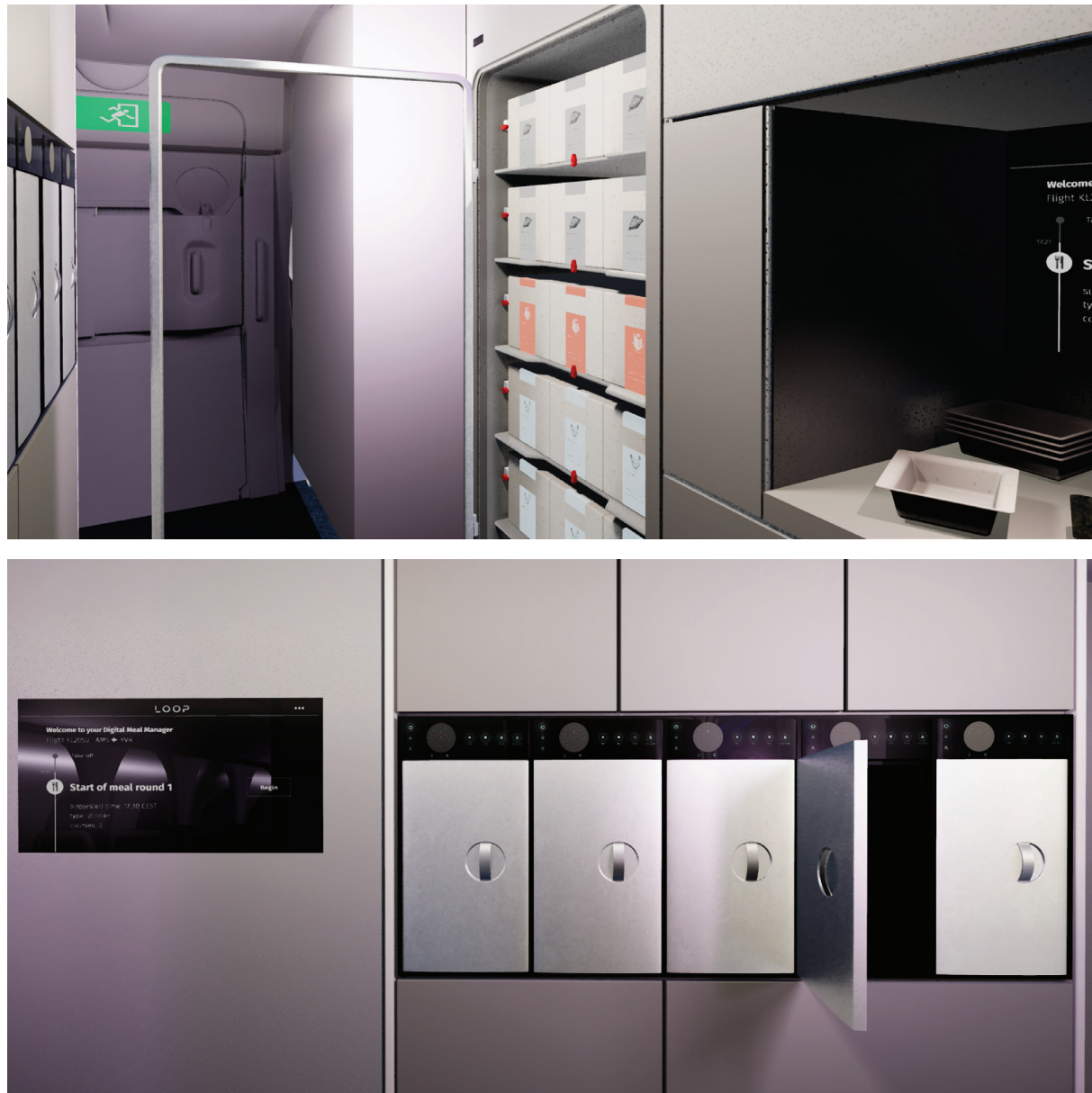
Figure 31 The kitchen galley located in area D. The door of the fridge can be opened by the 'player' in virtual reality, as well as the doors of the ovens. A permanent screen is added next to the ovens, which is otherwise unused wall space. With that, the crew has access to the digital system to coordinate the onboard services.
