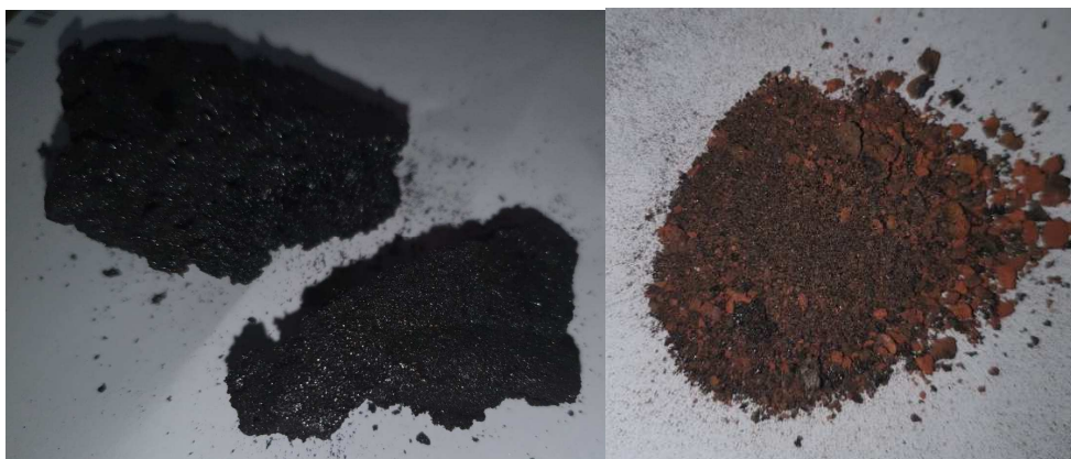
figure 54 (left) The char with an ash content of 11.0 m% that was deposited in the reactor chamber at low temperature (<500 °C) operation with low equivalence ratio (<0.25) and high S/F ratio ( \geq 0.58 ). (right) The leftovers of the char after heating the sample up to 850 °C with a fresh air supply. The red color could indicate a high concentration of iron in the char.
