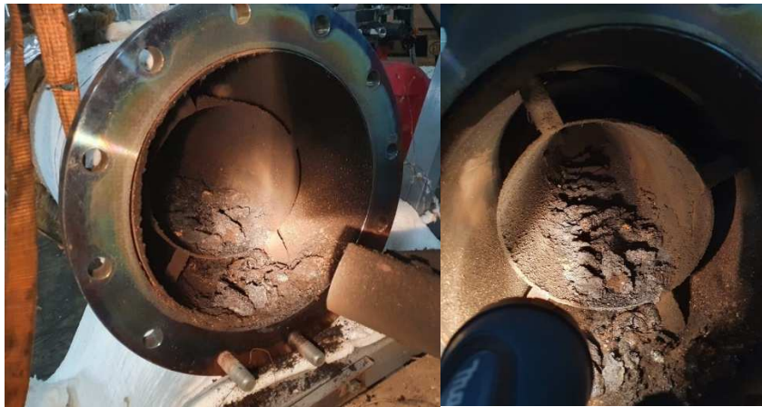
Figure 46 Char deposit with an ash content of 11.0 m% in the reactor tube after operation at low temperature below the end of the boiling curve (566 °C)
