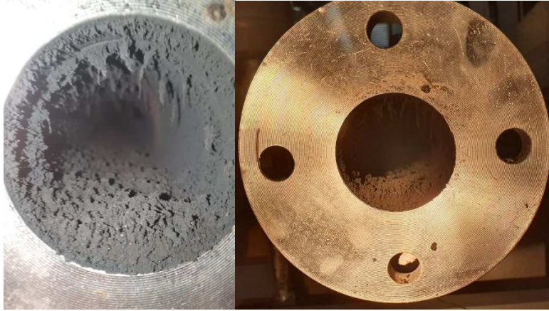
figure 47 (left & right) Heavy soot deposition in the 60 mm recirculation tube with an ash content of 2.42 m%
