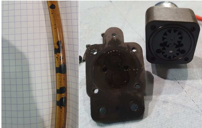
figure 53 (left) Tubing with tar deposition visible after operation with DKR350 pyrolysis oil and after flushing with diesel. (right) A broken oil pump used in the experiments which got clogged with the tars from the DKR350 pyrolysis oil
