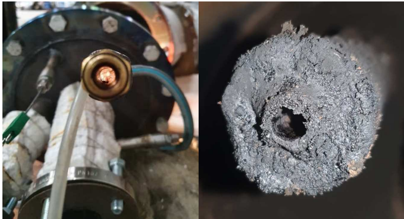
figure 52 (left) Look-through to the oil injection tube showing a clean tube after operation indicating no charring inside the oil injector lance. (right) Heavy charring on the outside of the water cooled oil injector lance, however the outlet of the oil injector is clean
