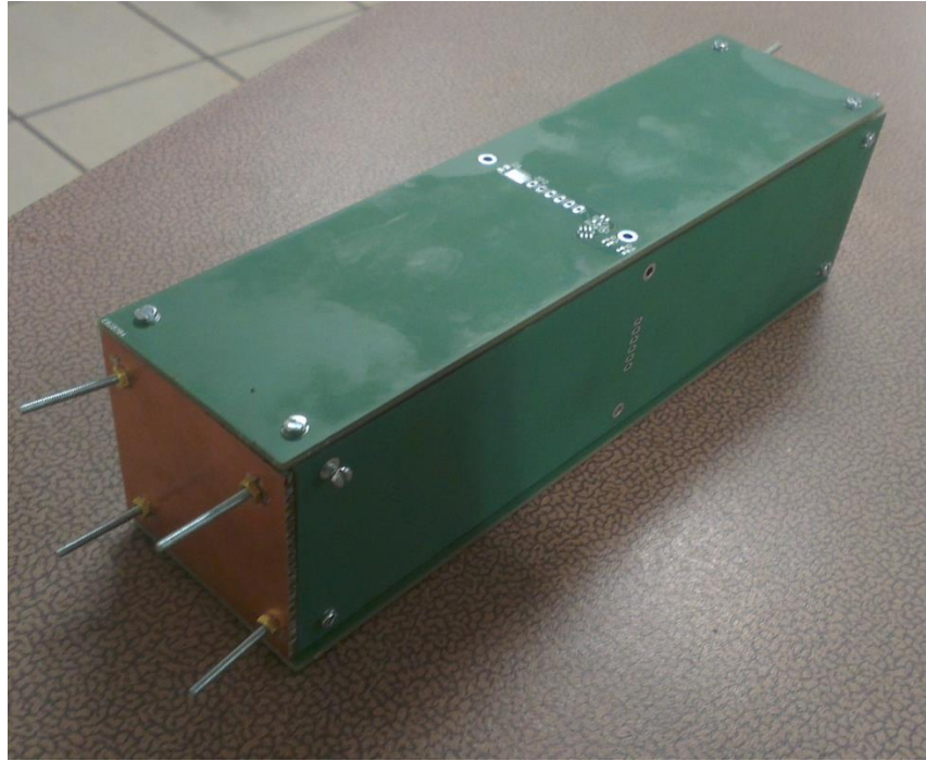
Figure 64 PCB outer structure example prototype.
