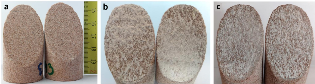
Figure 3. Pictures of (dried) samples before (a) and after the experiment was finished (b and c). Note that the tips of the saw-cut are ground off <3 mm, but the overall shape is still elliptical, with dimensions [45 \pm 0.7 \text{ mm}/29.6 \pm 0.1 \text{ mm}] . The middle (b) shows a sample after stepwise injection and the right (c) after cyclic injection. The formed gouge is visible as the patchy whitish powder on the saw-cut fault surface. The patterns of final gouge distribution were different after each experiment, without any relationship to experimental parameters.
