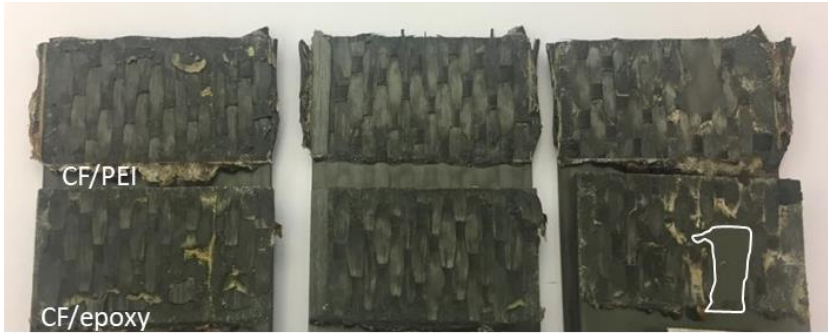
Figure 2.14: Fracture surfaces obtained from ED-less-250 samples welded at 600 J. Unwelded areas are indicated by the white lines. White arrows indicate locations with discoloured PEI resin.
