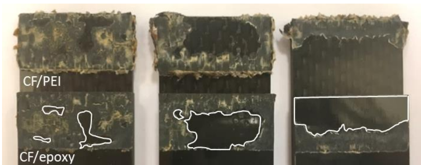
Figure 2.12: Fracture surfaces obtained from ED-less-60 samples welded at 500 J. The white lines indicate the unwelded areas.
