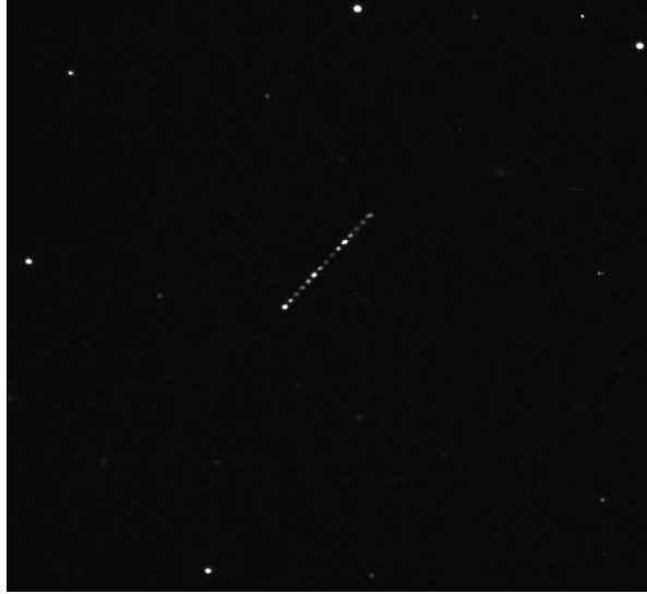
Figure 2.2: Stack of 15 images taken with the 0.51-m telescope of MPC Q65 Warrumbungle, Australia, on 11 September 2015. Note the the slow brightness variation with periodic specular peaks in brightness. Image courtesy M. Langbroek
