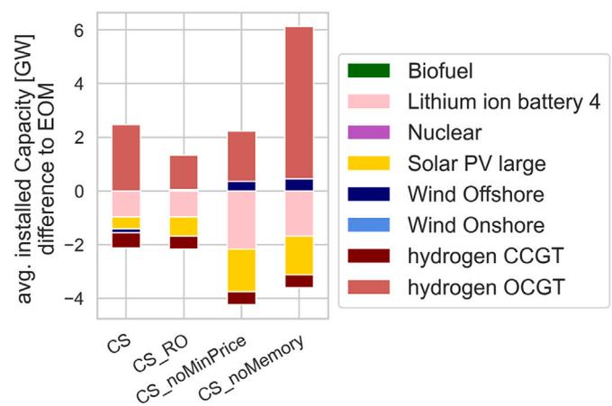
Fig. 15. Difference in the average installed capacity in 10 last simulation years between the CS scenarios and an EOM.
