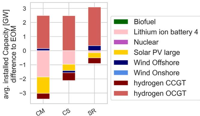
Fig. 22. Difference in the average installed capacity over the last 10 simulation years between CRM scenarios and an EOM.
