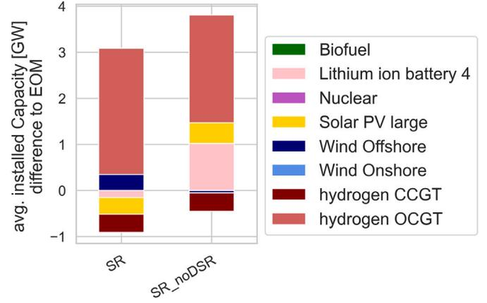
Fig. 9. Average difference of installed capacity in 10 last simulation years with SR scenarios. Without DSR prices were more volatile which incentivized more batteries.
