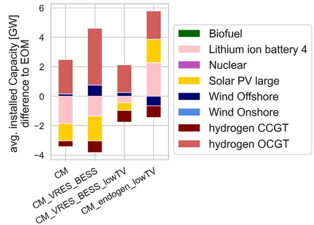
**Fig. 5.** Difference in the average installed capacity over the last 10 simulation years between the CM scenarios and an EOM. In all CM scenarios, the installed capacity of H<sub>2</sub>-turbines increased.
