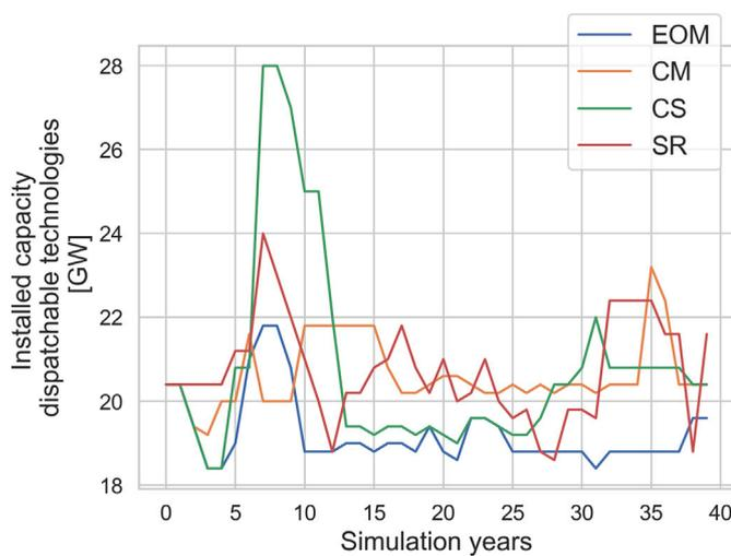
Fig. 20. Yearly installed capacity of dispatchable technologies which include nuclear, bioenergy, and H<sub>2</sub> turbines.
