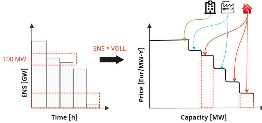
**Fig. 3.** For each consumer group, the hourly energy not supplied, per blocks of 100 MW, determines the volume-price bids. In this way, we simulate consumer groups assigning different values to parts of their load. For example, households might value lower their EV load. The demand curve is then the aggregation of all consumers' segmented bids.
