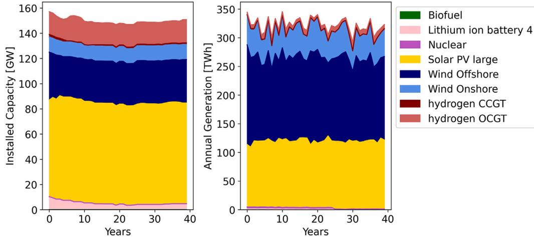
**Fig. 4.** Left: Installed capacity per technology in an EOM. Solar energy was the technology with the highest installed capacity. Right: Annual generation per technology in EOM. The annual production of wind energy was volatile year-to-year.
