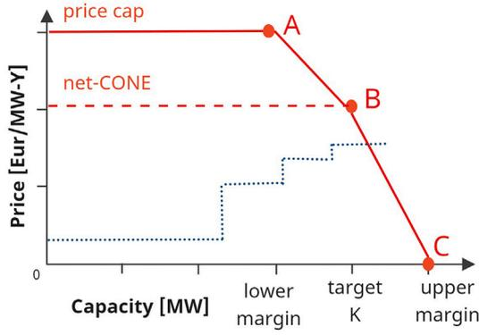
Fig. 2. Sloped demand curve in our simulations considering a centralized capacity market.
