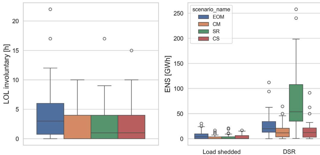
Fig. 19. LOLE and ENS by CRM. The mechanisms reduced the shortages to a similar LOLE and ENS. However, the activation of the DSR was much higher in an SR.
