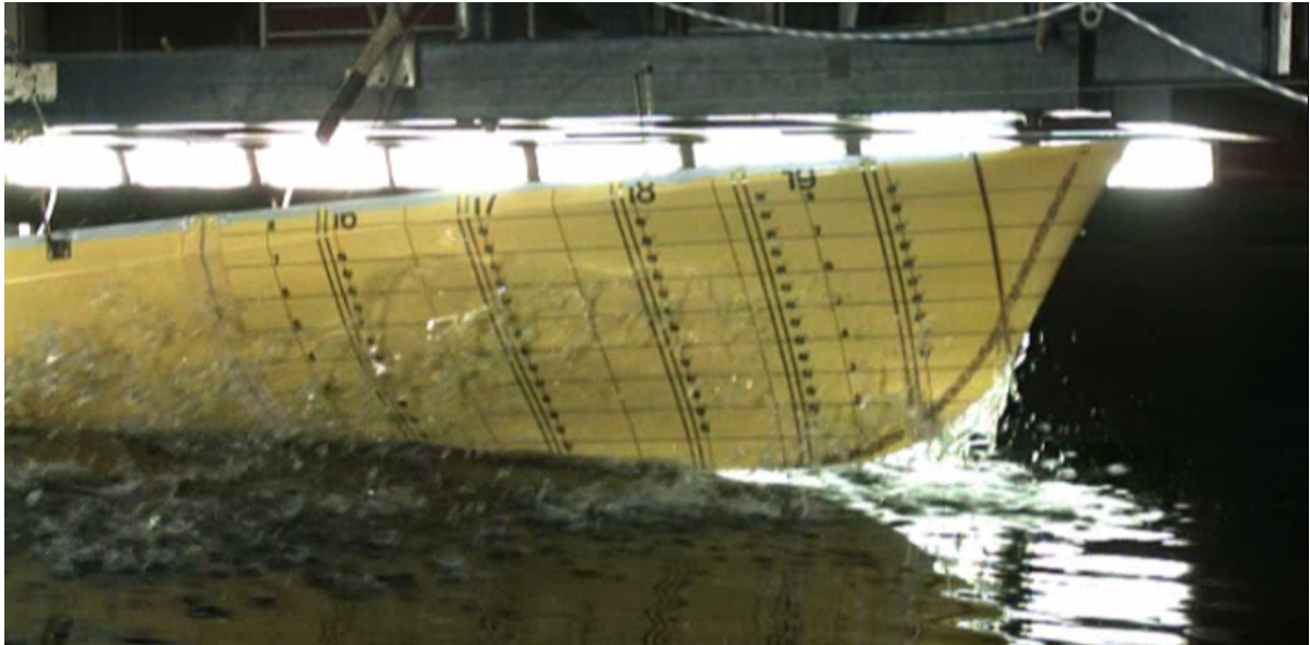
Figure 5.5: CRS model test footage [11] - bow lifting out of the water
