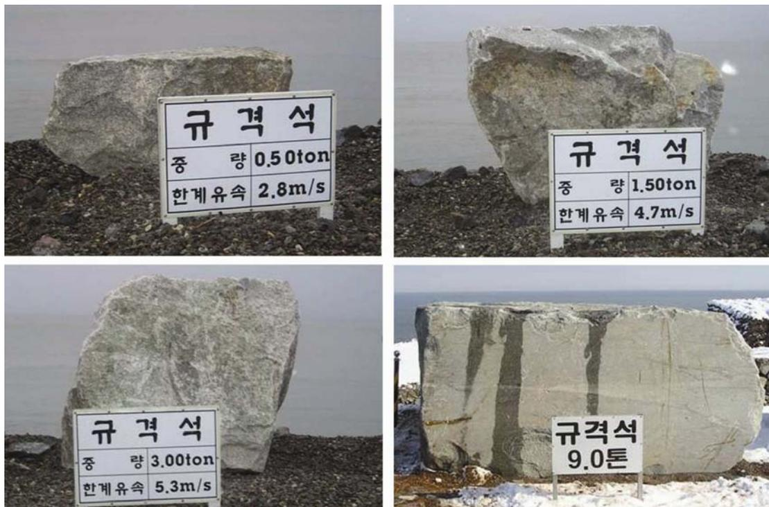
Figure 2-14 Different size of rocks used for the closure
