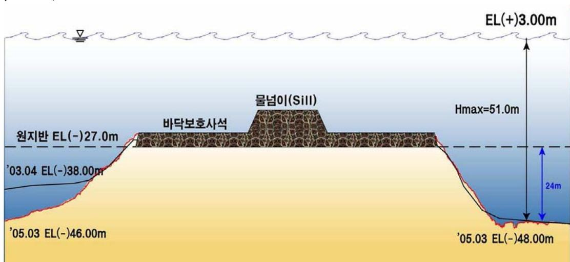
Figure 2-8 Cross section of a closure gap with scour holes and bottom protection
