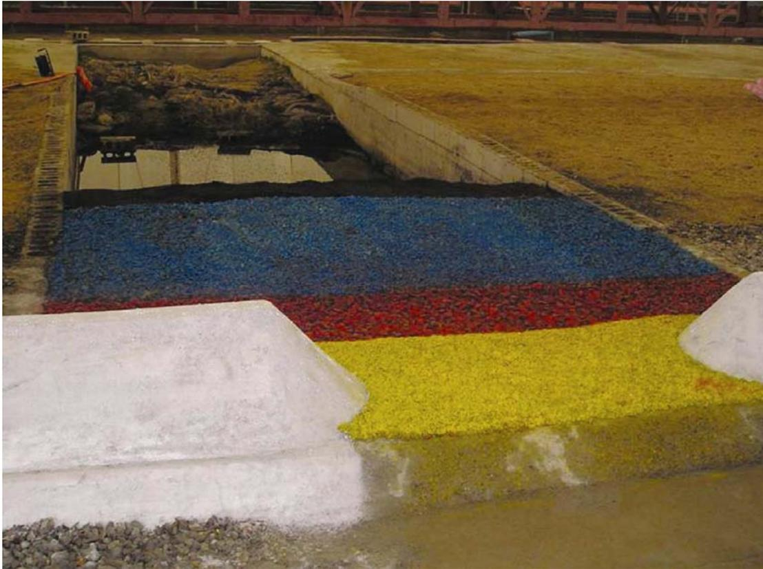
*Figure 2-5 Detailed scale model for testing gabion behaviour*
