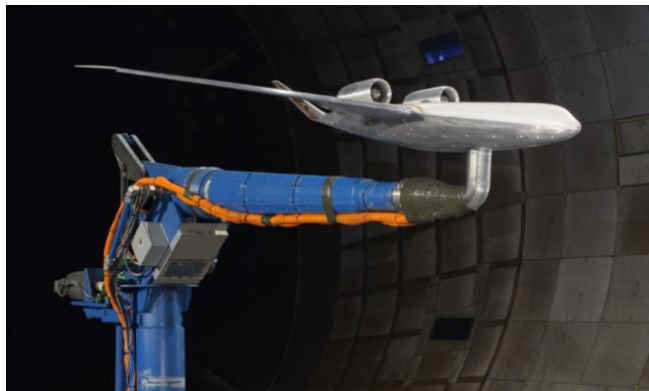
(a) Photo of the NASA/Boeing BWB design in the NFAC 40x80 Foot wind tunnel 9
