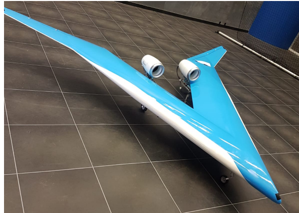
(c) The Flying V SSFT model (without winglets) sitting on the floor of the wind tunnel
