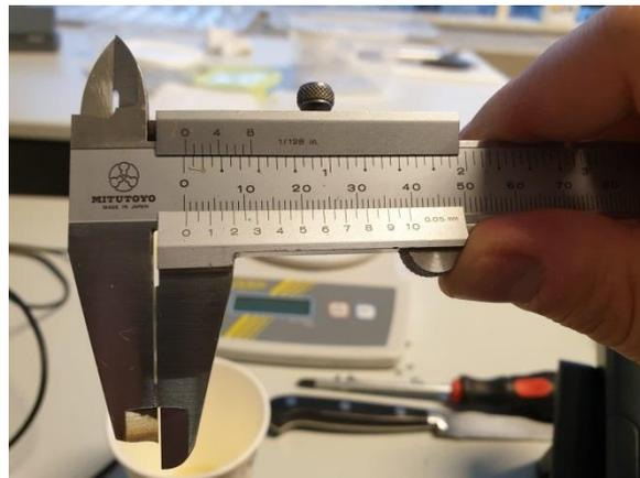
Figure 20: Thickness of die of other participant measured using caliper.
