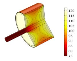
Figure 6 Stationary temperature distribution within the SPP based on estimated heat transfer coefficients.
