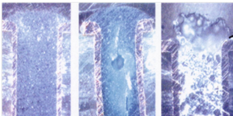
Fig. 4.25 Cross sections of vias after thermal cycling (condition B: -55 to 125 °C, liquid/liquid immersion, 10 min cycles)
