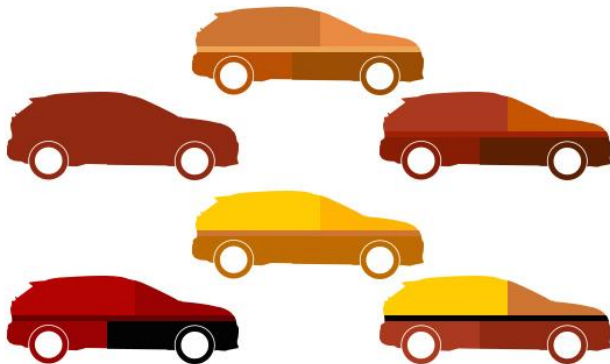
Figure 4.17: A wide range of vehicles can be developed, by designing and using efficiently a smaller well of standardized segments (derived by Renault Group, 2016)
