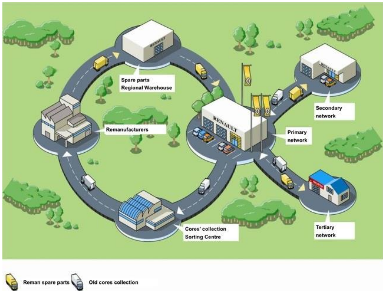
Figure 2.20: The damaged parts (scraps) from vehicles in use are being collected through the commercial reverse logistic network.
