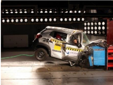
Figure 4.7: Prototype vehicle is getting tested against frontal collision (Function testing).
