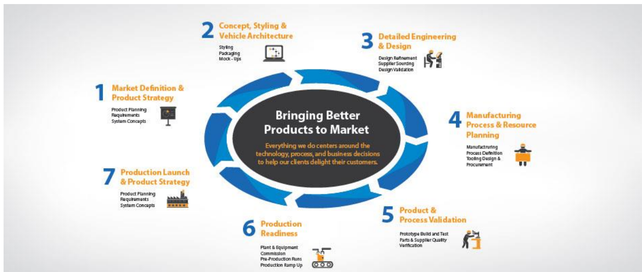
Figure 4.2: The steps of introducing a new car in the market (source: Tata technologies web site)
