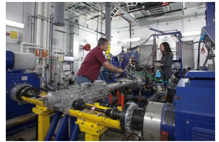
Figure 4.9: Manual transmission durability testing, supplemented by exhaustive testing i Milford and state-of-the-art laboratories in Pontiac, Michigan
