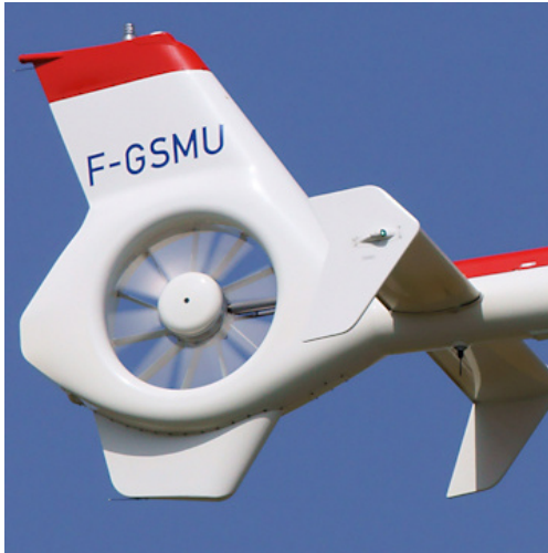
Figure 1.3: Fenestron tail, Eurocopter EC-135
