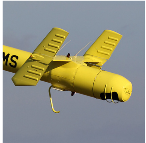
Figure 1.4: NOTAR System, MD Explorer
